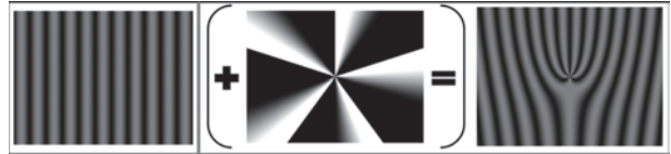
Figure 5. Left side: numerically generated matrix plot of two interfering plane waves, which results in a diffraction grating that can be used to holographically diffract a normal, l = 0 beam. Right side: Similar situation, except now one of the interfering plane waves used to construct the grating is imposed with a spiral phase of e^{il\phi} for l = 5 (center); this creates a forked diffraction grating (right), which will holographically generate a Hypergeometric-Gaussian (HyGG) mode with l = 5 in the first diffracted order.
