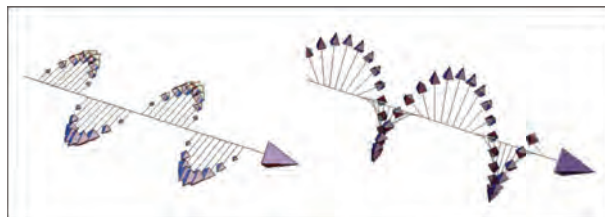
Figure 1. The arrows represent the electric field of a propagating beam. Light with no SAM is linearly polarized (left) and light with SAM is circularly polarized (right). Figure from 1 .
