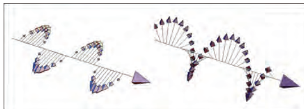
Figure 1. The arrows represent the electric field of a propagating beam. Light with no SAM is linearly polarized (left) and light with SAM is circularly polarized (right). Figure from 1 .
