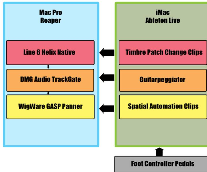
Figure 2 GASP signal routing overview across Mac Pro and iMac. Copyright 2019 by E. Fitzmaurice.
