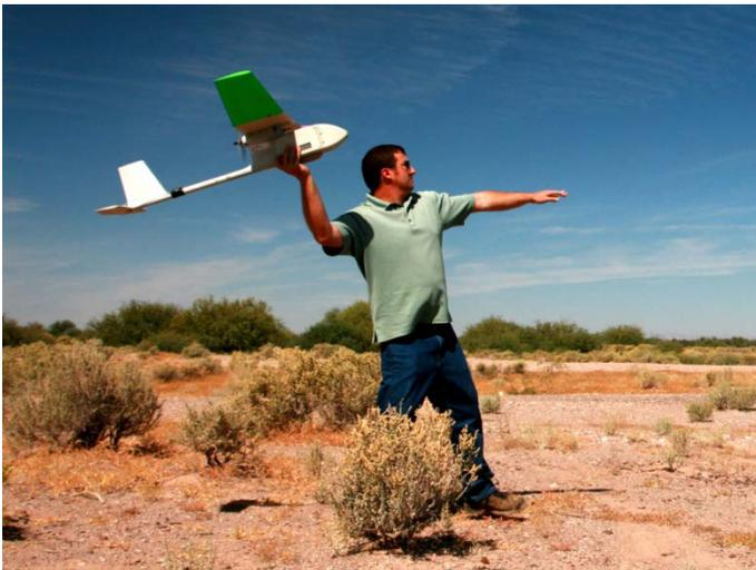
Figure 1: Raven-RQ-11a is launched by hand on BLM lands.
