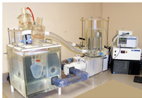
Figure 7. Left – DU pulse duplicator system; Right – valve prepped for testing in a washer to be mounted in the pulse duplicator.
