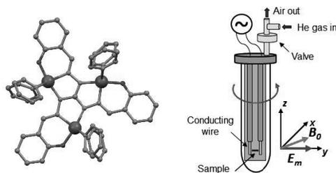
**Fig. 1** Left: the molecular structure of the spin-frustrated Cu<sub>3</sub>, with a total ground state S=1/2. Right: schematic view of the modified version of the sample holder used for the EFM-EPR measurements. The electric field ( $E_m$ ) is obtained by applying an alternating voltage  $V = V_0 \cos(\omega t)$ , with  $V_0 = 170$  V over a distance of 1.5 mm, and  $\omega = 2\pi \times 30$  kHz.
