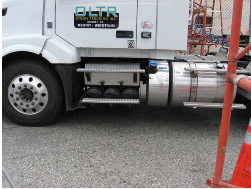
Figure 4. Driver side image of a HDV with the urea tank clearly visible.
