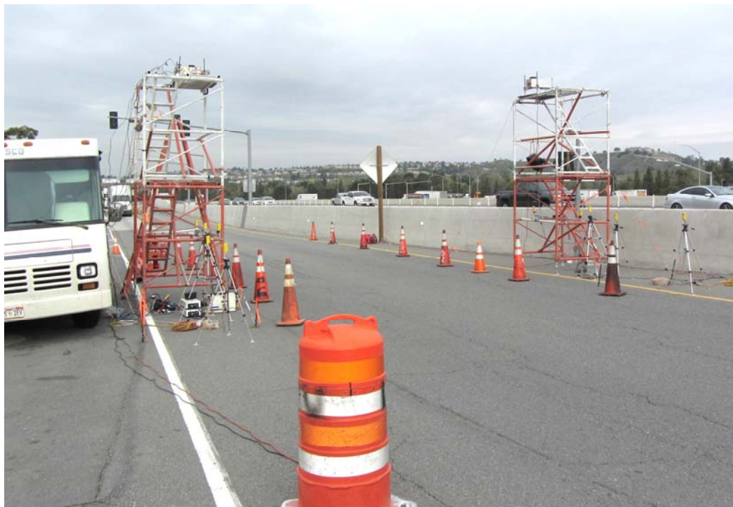
Figure 1. Photograph at the Peralta Weigh Station of the setup used to detect exhaust emissions from heavy-duty diesel trucks.
