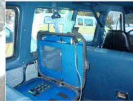
The compact emission analyzer was carried inside the vans and a hose run out to the exhaust pipe. Researchers traveled with the equipment.
