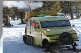
The oldest snow coaches are Bombardiers. Most have older carbureted engines that have high emissions.
