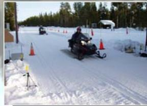
Snowmobiles emissions were measure on entry and exit. One sled was instrumented for direct exhaust emissions measurements.
