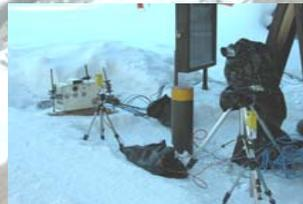
Above is part of the remote sensing equipment used at the West gate to measure snowmobile emissions. The snowmobile below is just going through the IR-light beam.
