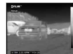
Both of the vehicles in the IR images above are hot, however because snow does not reflect IR radiation, there is no reflection on the road from the underbody of the vehicles.
