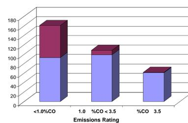
This graph shows the number of vehicles that received a GOOD, FAIR, or POOR rating, as well as if the vehicle was a cold or hot vehicle. Only one vehicle received both a POOR rating and was a hot vehicle from both days of measuring vehicles at the high school.
