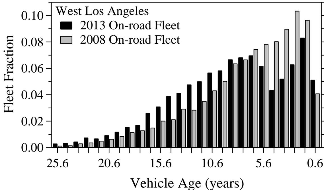
**Figure 3.** Comparison of on-road fleet fractions versus vehicle age in years for the last two data sets collected at the West Los Angeles site. The black bars are the current data set collected in April/May of 2013 and the grey bars were collected in March of 2008. Vehicle age was calculated assuming that new vehicle model years begin in September and as a result the newest vehicles (0.6 yrs old) represent model years 2013 and 2008 respectively.
