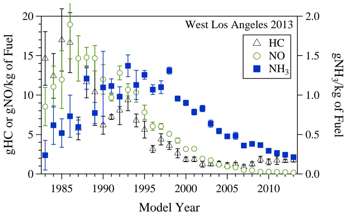
**Figure 4.** Fuel specific emission factors for HC, NO (left axis, open symbols) and NH<sub>3</sub> (right axis, filled squares) versus model year for the 2013 West Los Angeles data. Errors plotted are standard errors of the mean determined from the daily means.
