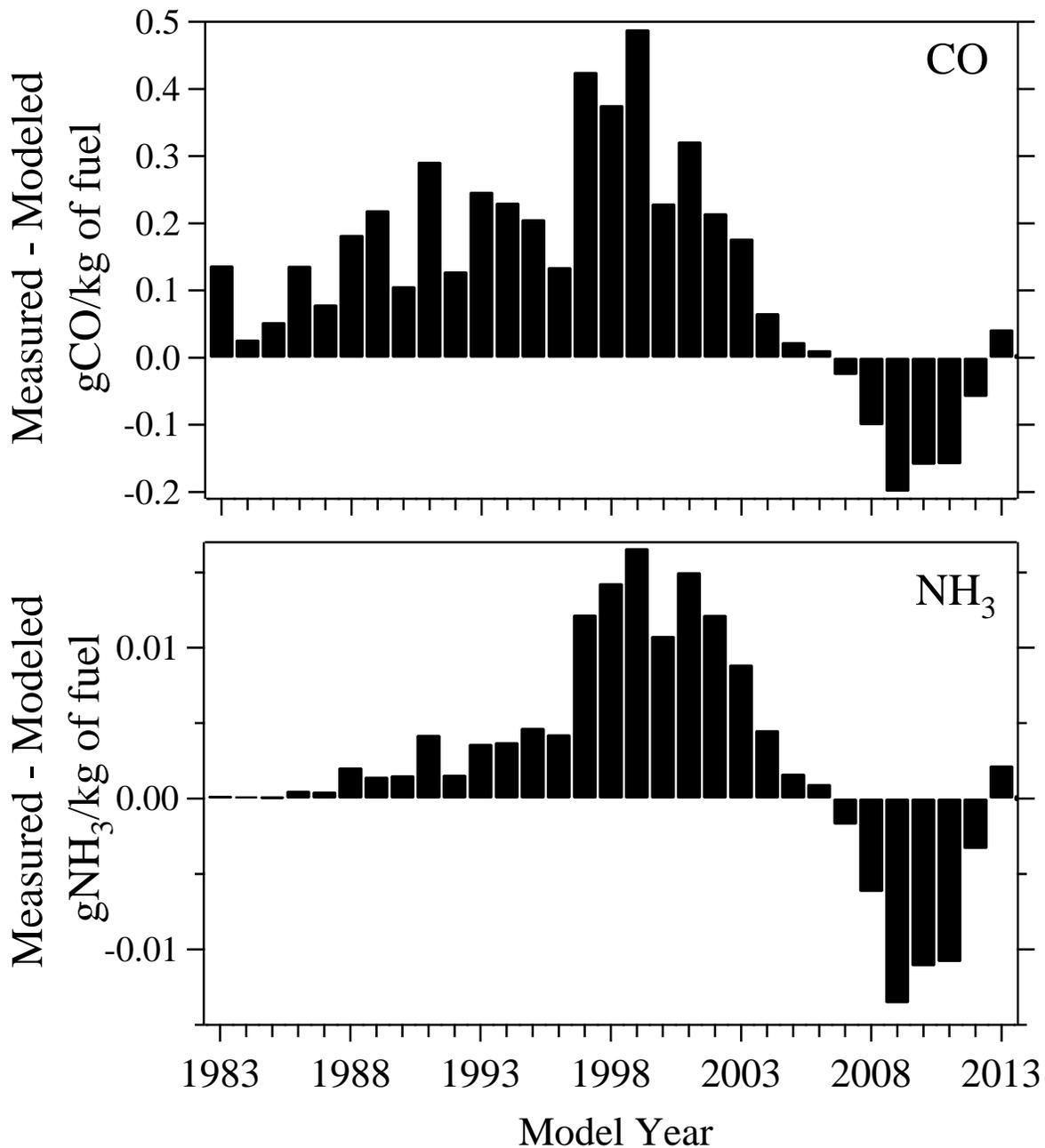
**Figure 5.** Measured minus modeled g/kg of fuel emission differences from Table 2 (3.9 g/kg of fuel for CO and 0.08 g/kg of fuel for NH<sub>3</sub>) distributed by model year for the 2013 West Los Angeles data set. Positive values indicate 2013 emissions that would not be present if the rate of fleet turnover had not been slowed by the recession and the 2013 fleet’s age distribution was as measured in 2008. Negative values are model years where emissions are lacking due to fewer vehicles.
