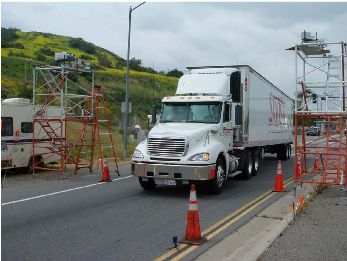
**Figure 1.** Photograph of the emissions sampling setup at the Peralta weigh station site. Shown on top of the scaffolding are a commercial remote sensing unit (on the left) and the University of Denver’s FEAT multi-species remote sensor (on the right). The speed sensing units are mounted in the middle of the orange scaffolding section. The data acquisition computers and calibration cylinders are contained in the motorhome at the left.
