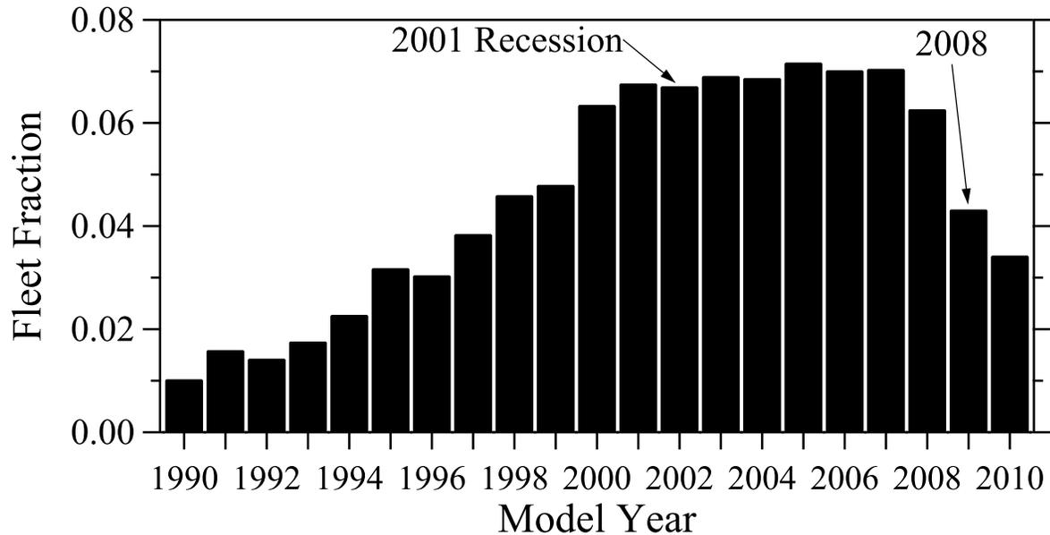
**Figure 1.** The measured Sherman Way fleet fraction versus model year for 1990 and newer models. The 1989 and older vehicles make up 3.5% of the total fleet. The 2001 recession is not detectable in this data set, while the 2008 downturn is quite striking in its magnitude and has rapidly aged the vehicle fleet.
