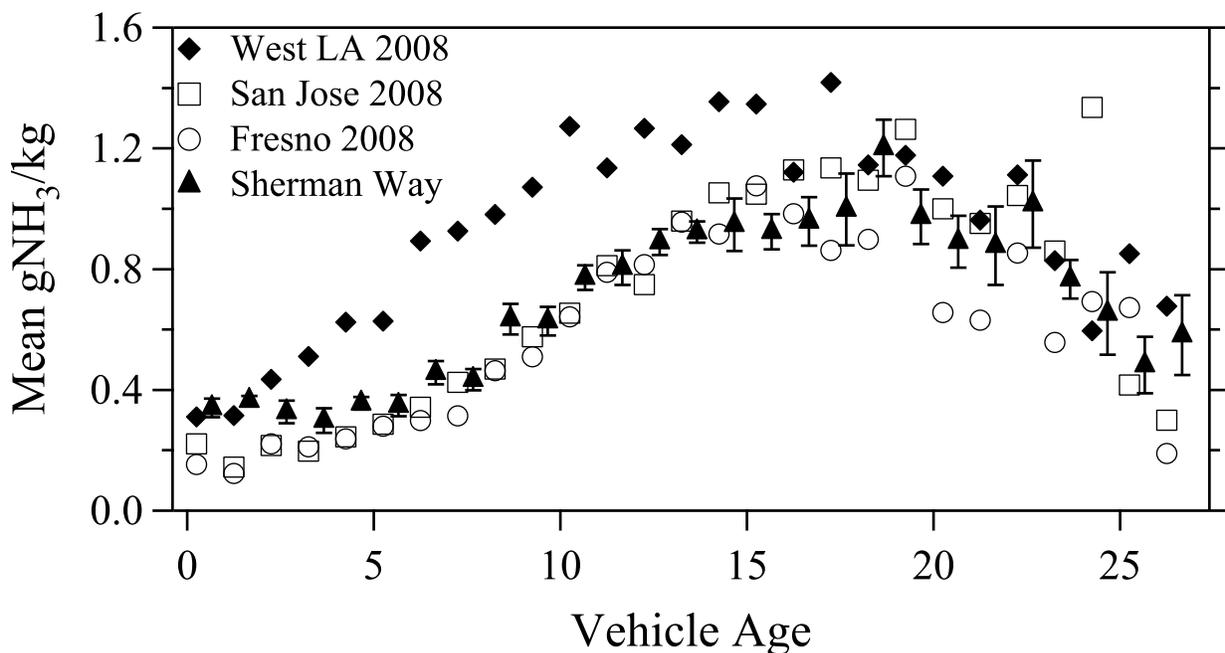
**Figure 3.** Mean  $\text{gNH}_3/\text{kg}$  emission versus vehicle age for the Sherman Way data (filled triangles) compared to three California sites measured in March of 2008. Vehicle age has been defined as the difference between the fractional measurement year and the vehicle model year. The error bars plotted are standard errors of the mean calculated using the daily model year means and all of the emission values have been calculated assuming a fuel carbon fraction of 0.85.
