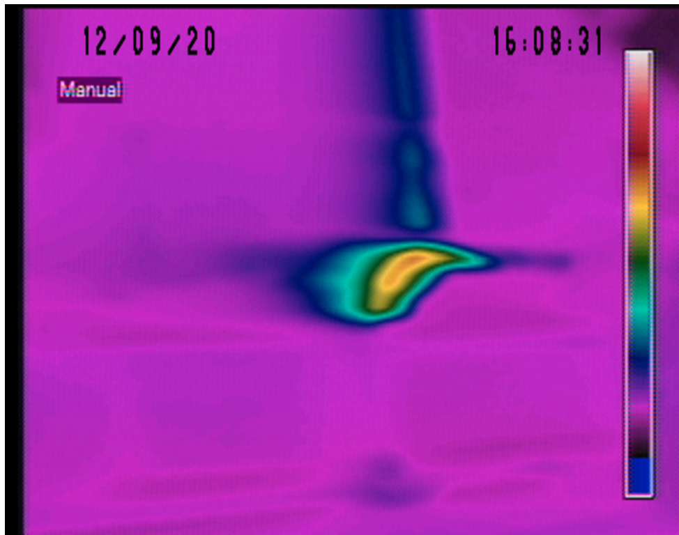
Figure S6. A thermal image of a truck with an elevated exhaust pipe collected on December 9 th . Pipe temperature was estimated at 115° C for this truck.
