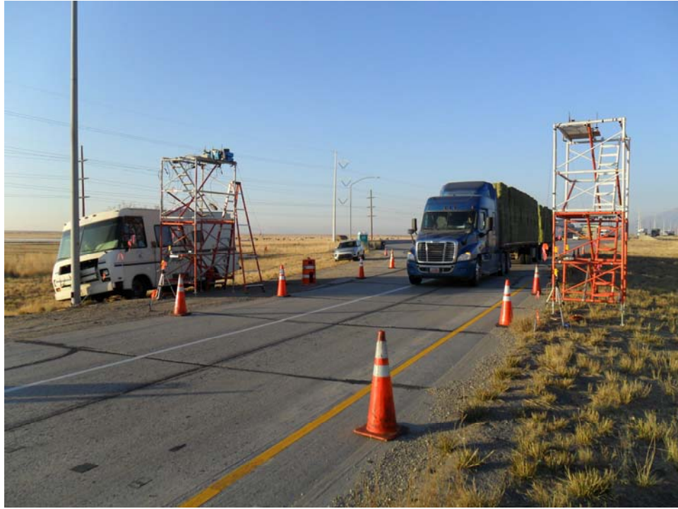
Figure S4. A photograph showing the scaffolding setup for measuring exhaust from trucks with elevated pipes. The light source is on the right tower and the detectors on the left. The road barrel on the far side of the highway houses the IR camera.
