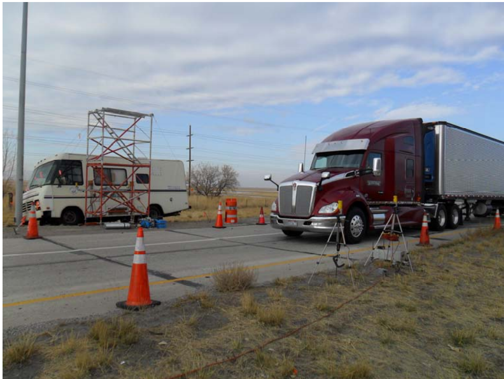
Figure S5. A photograph showing the ground level setup and the twin tripod mounted sensors used for measuring vehicle speed and acceleration.
