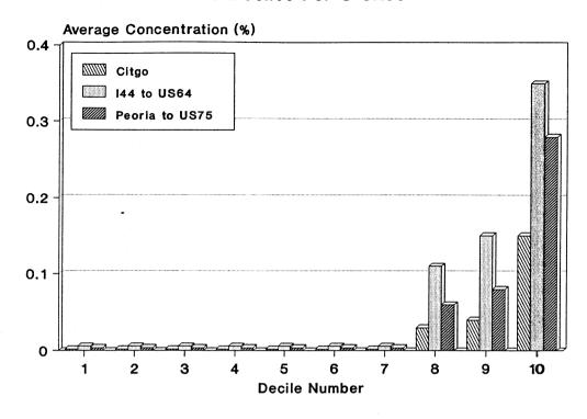
Figure 8. A histogram illustrating the average % HC emissions for each decile of the fleet at each site. Note that 70% of the vehicles at all sites have negligible emissions.
