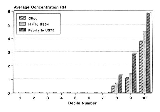
Figure 7. A histogram illustrating the average % CO emissions for each decile of the fleet at each site. Note that 70% of the vehicles at all sites have negligible emissions.
