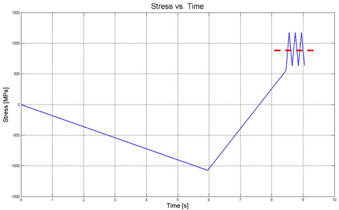
Figure 4.7 Stress vs. Time at element of interest for existing installation process (mean stress is designated by the dashed line)
