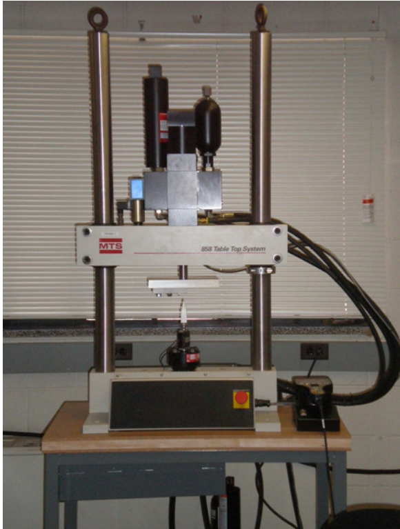
Figure 2.3 MTS 858 table top hydraulic test frame
