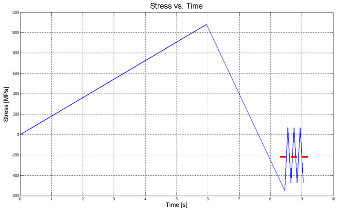
Figure 4. 11 Stress vs. Time at element of interest for modified installation process (mean stress is designated by the dashed line)
