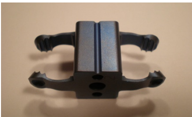
Figure 2. 2 StenoFix fatigue Specimen with all four wings plastically deformed
