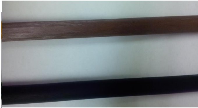
Figure 3-1. Aged ACCC core samples. As received (top) and coated (bottom).
