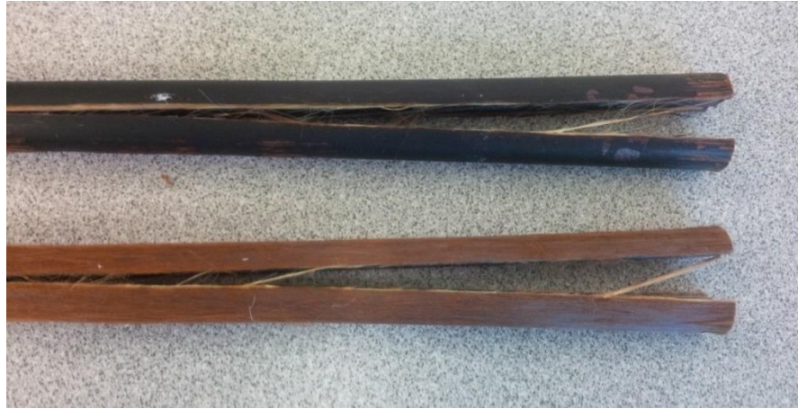
Figure 2-8. 12 month aged rods after flexural failure. Coated (top) and uncoated (bottom).
