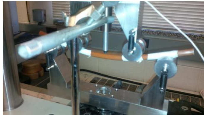
Figure 2-3. Four-point bend test apparatus.
