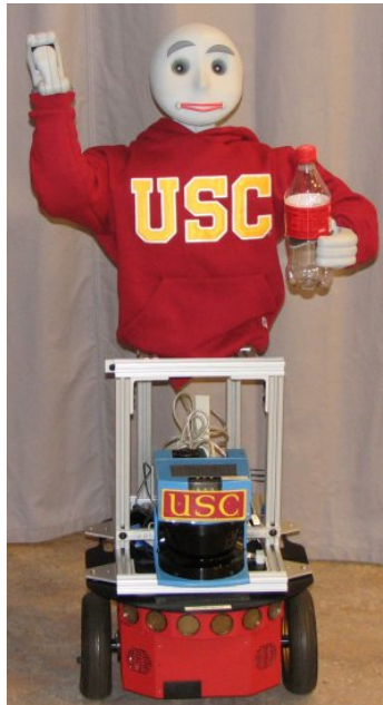
Figure 2.3: Bandit - A humanoid upper-torso robot of University of Southern California
