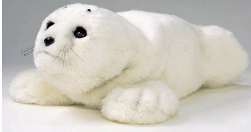
Figure 2.1: Paro Robot - A seal-like interactive robot
