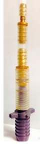
Figure 3.3.1 – Cannulated tubing structure to connect syringe for retrograde coronary flow towards the aorta. 1/3” diameter tubing for syringe insert was connected to 3/4” to 1/2” transition cannula which was further connected to 3/4” cannula that was secured into the aorta.
