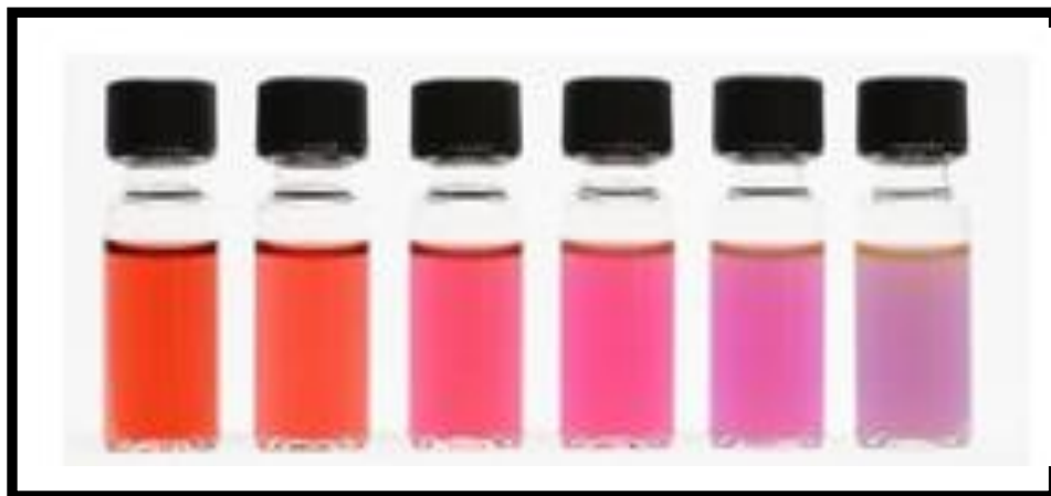
Figure 2.1: Size dependent colors of gold nanoparticles [36].
