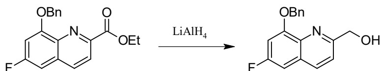
Scheme 2.3.15 Reduction of ethyl ester to hydroxymethyl using lithium aluminum hydride
