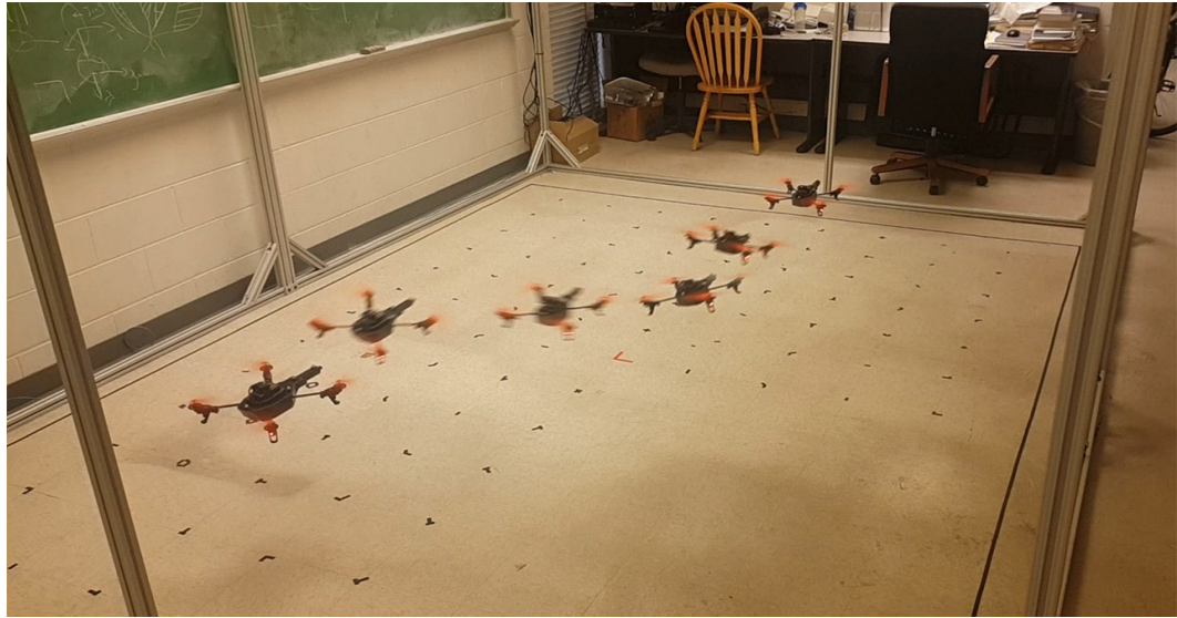
(a) The quadrotor is commanded to move towards a horizontally virtual moving obstacle.
