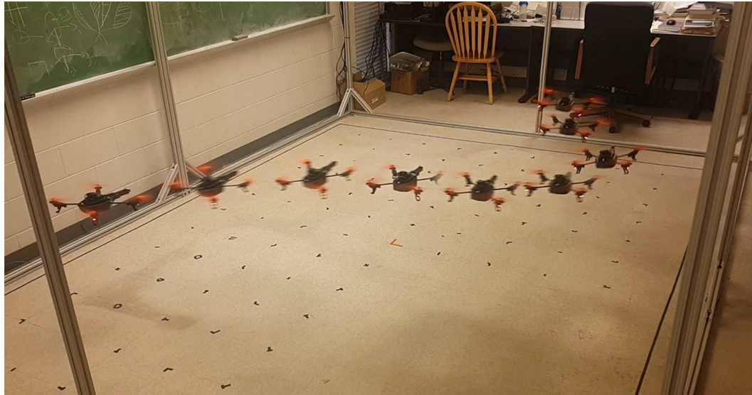
(a) The quadrotor is commanded to fly towards a diagonally virtual moving obstacle.
