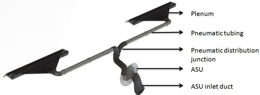
Figure 4.9: CAD model of the CC system [8].
