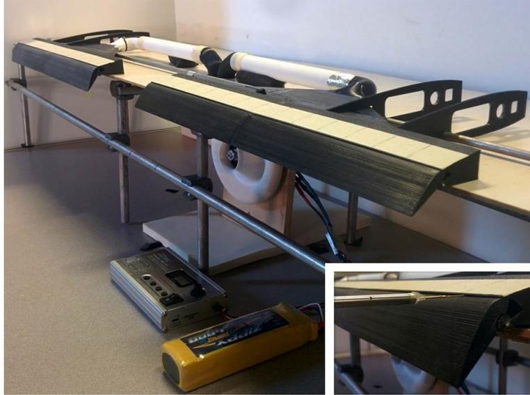
Figure 4.10: The experimental setup of the CC system.
