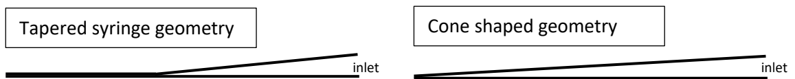
Figure 40. The tapered syringe design and the cone shaped nozzle geometry, each with same inlet and outlet dimensions
