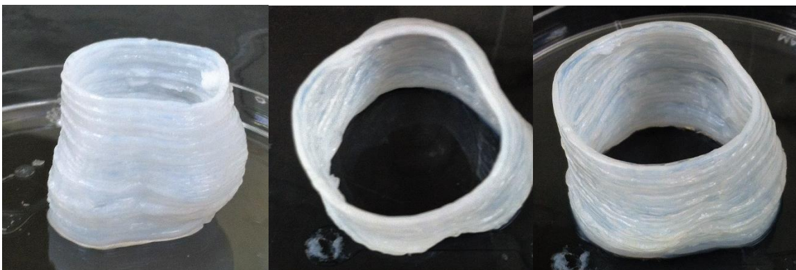
Figure 67. Thin walled scaffold printed with thickness between 0.4mm-0.8mm, and dimensional fidelity is +/- 2% with several dramatically overhung features. Gelatin 5% -PEGDA 15% w/v copolymer.
