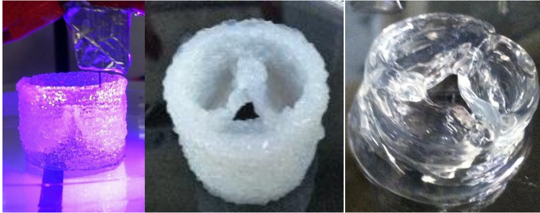
Figure 70. Aortic valve scaffolds from early testing with testing with alginate-PEGDA copolymer hydrogels.
