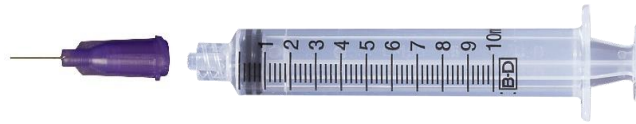
Figure 35. BD 10ml syringe and Jensen Global 0.21mm I.D. nozzle used. Jensen dispensing tips feature a polypropylene Luer Lock hub with a UV-bonded 304 stainless steel cannula.
