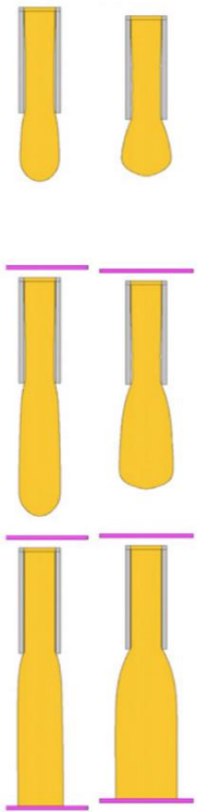
Figure 75. The Barus effect changes the cross-sectional area as flow leaves the nozzle, slowing its average velocity and affecting the print settings 6 .
