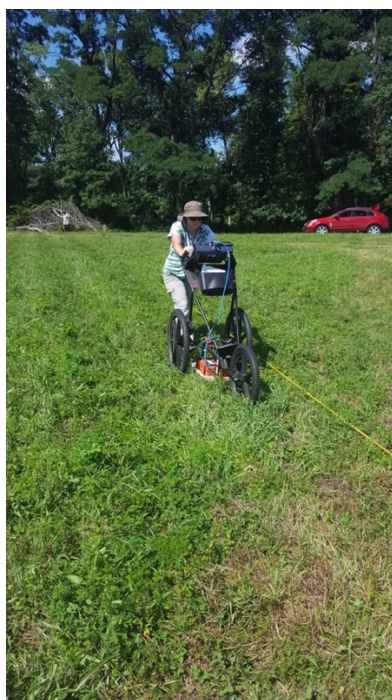
Figure 3.12: Maeve Herrick collecting Grid 2. The 400 MHz antenna is the orange box being pushed along the ground. It is connected to the SIR 3000 control unit with a blue
