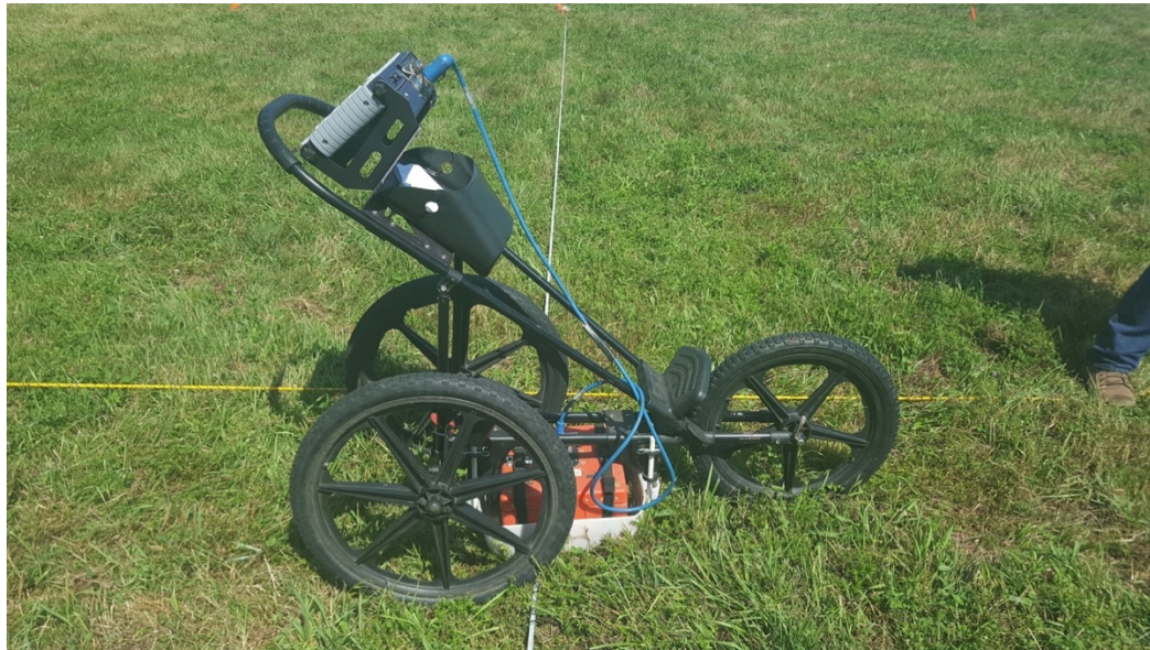
Figure 3.7: The GSSI 400 MHz antenna is the orange box attached to the bottom of the cart. The blue cord connects the antenna to the GSSI 3000 control unit, where the data is stored.
