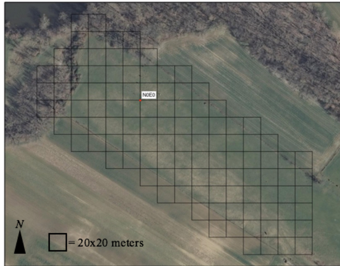
Figure 3.1: Image of the local grid that was established across the site. The red dot indicates the location of the N0E0 point, which is over a historical well. Each square in the grid is 20x20 meters. (Basemap from CTECO 2012).
