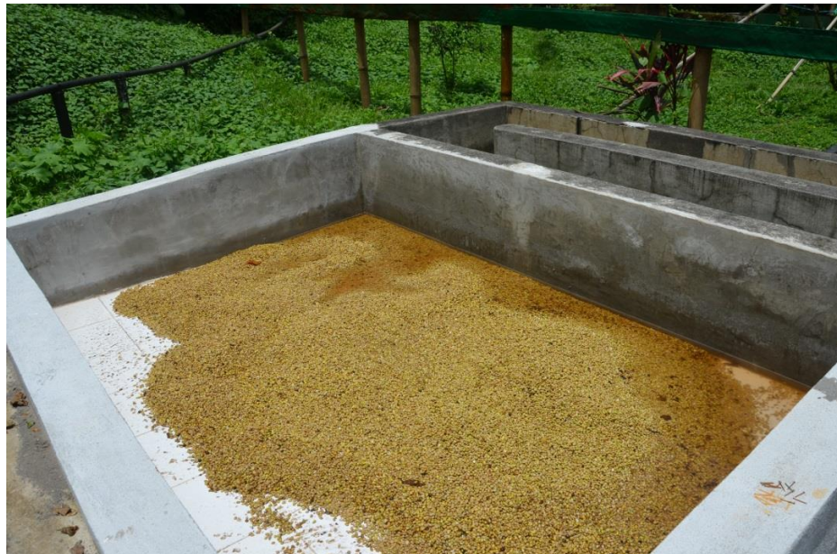
Figure 3.3. Fermentation tank used in the lavado processing of coffee. Source: Jessica Hook 2015
