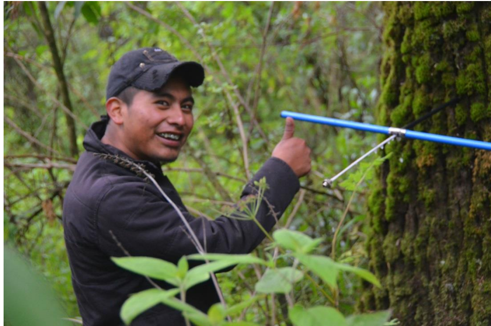
Figure 8. Fieldtrip in Kanchej forest, teaching a municipality forest trainee on the use of increment borers for dendrochronology studies.
