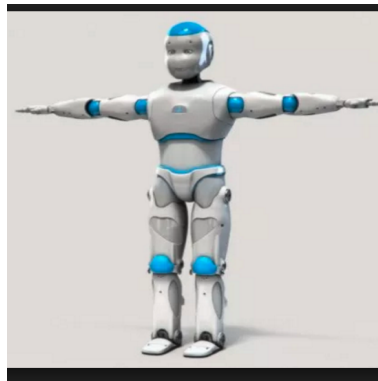
FIGURE 4.2: A Humanoid increasing its rotational inertia by spreading its arms alongside the Y-axis
