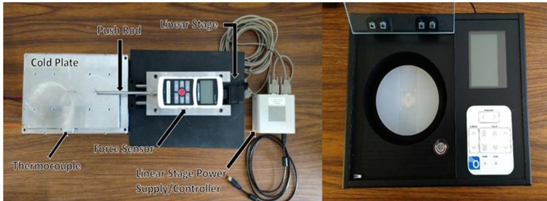
**Figure 22:** Cold plate with ice adhesion test apparatus (left) and spin coater (right).
