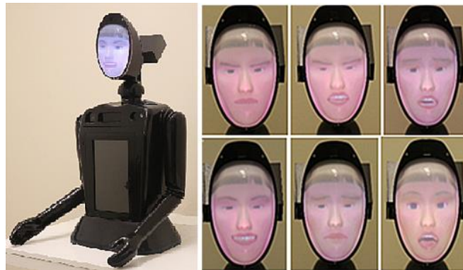
Fig 3-1 Left) Ryan Companionbot robot [31,32]. Right) Expressions demonstrated by Ryan with 100% intensity (Top from left to right: anger, disgust, fear. Bottom from left to right: happiness, sadness, surprise)
