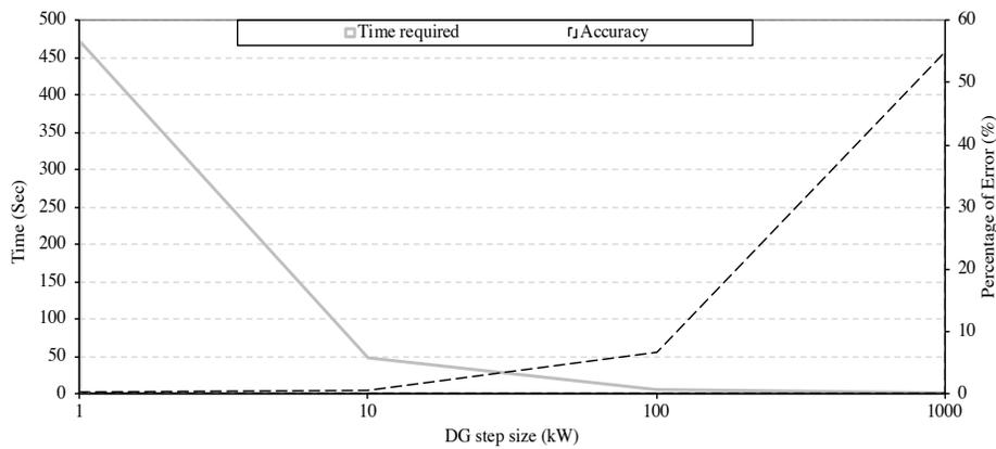
Figure 6.3: Tradeoff between speed and accuracy for each DG step size based on the iterative method.
