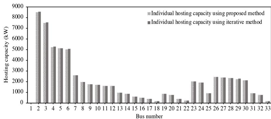
Figure 6.4: Hosting capacity for each individual bus (accuracy comparison).
