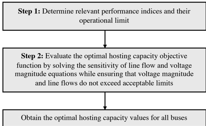
Figure 5.1: The proposed sensitivity-based hosting capacity method.
