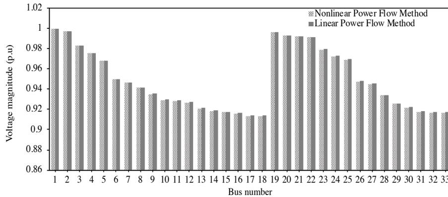
Figure 6.2: Voltage magnitude comparison between linear and nonlinear power flow methods.
