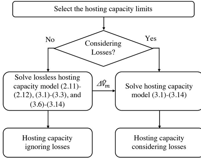
Figure 3.1: Flowchart of the hosting capacity calculation method.
