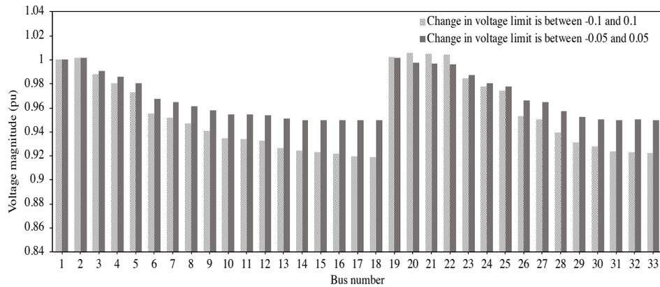
Figure 6.10: Voltage magnitudes based on hosting capacity results under base load conditions.
