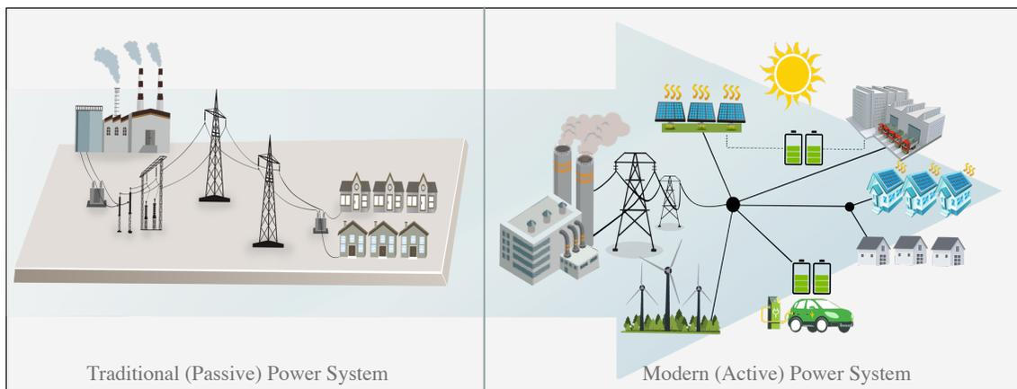
Figure 1.1: A comparison between traditional and modern grid topologies.
