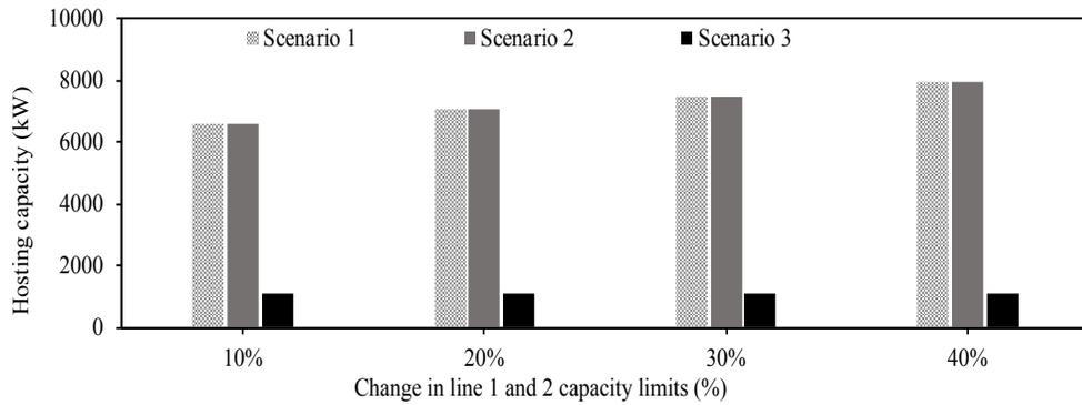
Figure 6.6: Hosting capacity results based on the change in capacity limits of lines 1 and 2.
