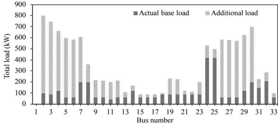
Figure 6.11: Fixed load and Additional load capacity for each individual bus.
