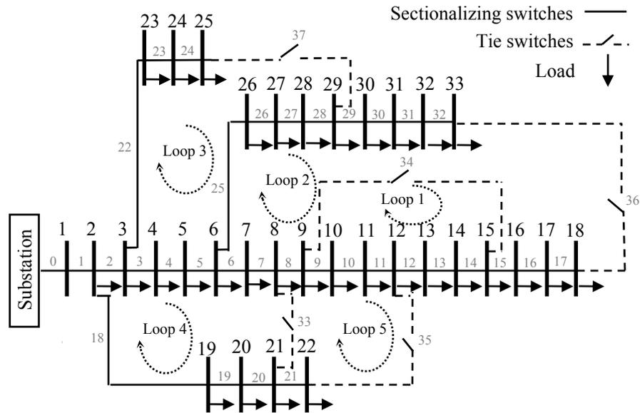
Figure 6.1: Single-line diagram of the IEEE 33-bus distribution test system.
