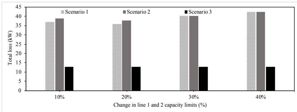
Figure 6.7: Line loss based on the change in capacity limits of lines 1 and 2.
