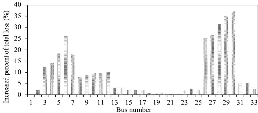
Figure 6.12: Total change in system losses when optimizing additional capacity in each bus.
