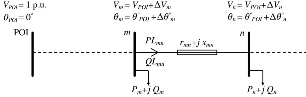
Figure 2.1: Representation of radial distribution lines.
