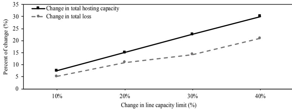
Figure 6.8: Change in hosting capacity and losses due to the change in capacity limits of lines 1 and 2.
