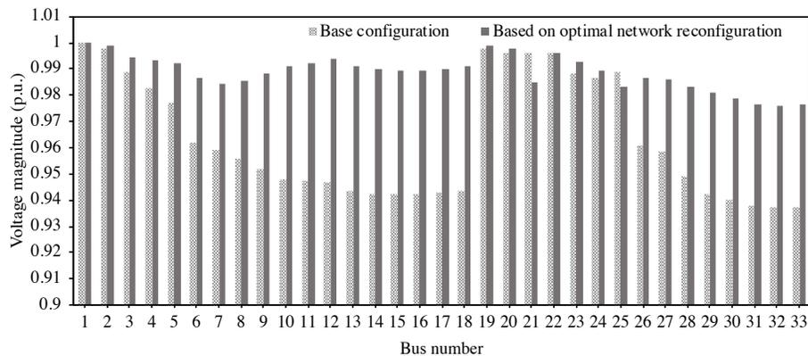
Figure 6.16: Comparison of the voltage profile with and without network reconfiguration.
