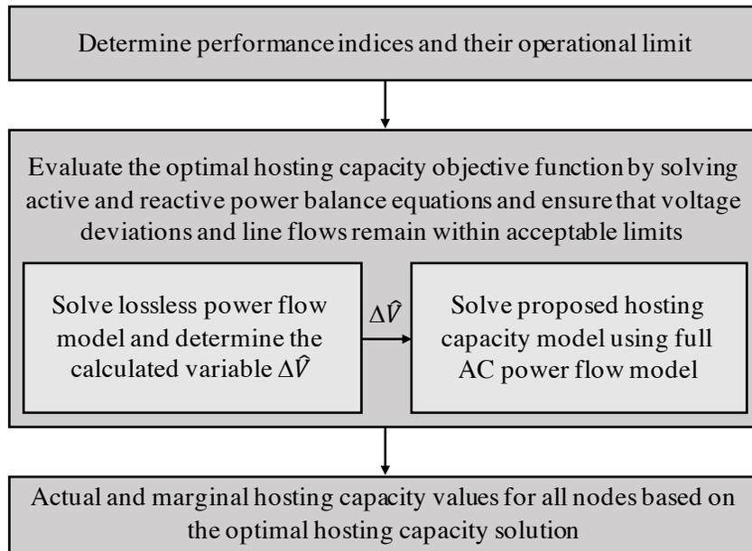
Figure 3.2: Proposed marginal hosting capacity calculation procedure.
