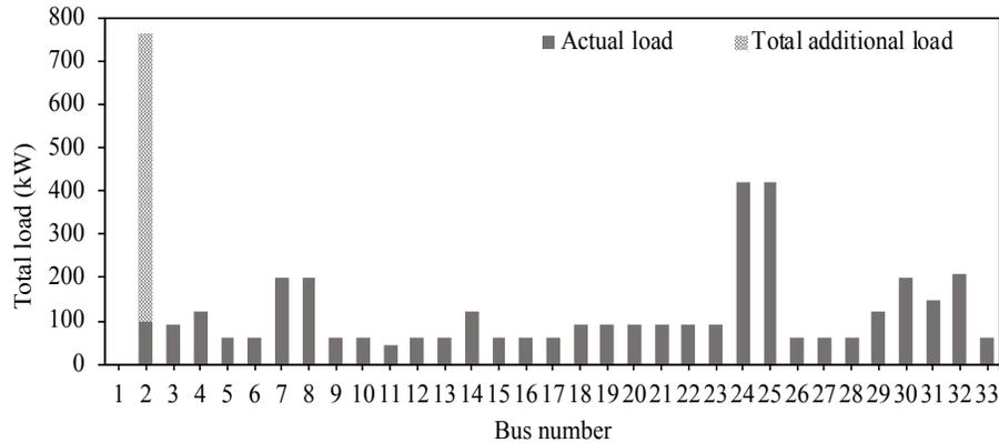
Figure 6.13: Fixed loading and optimal additional loading capacity when considering all buses.
