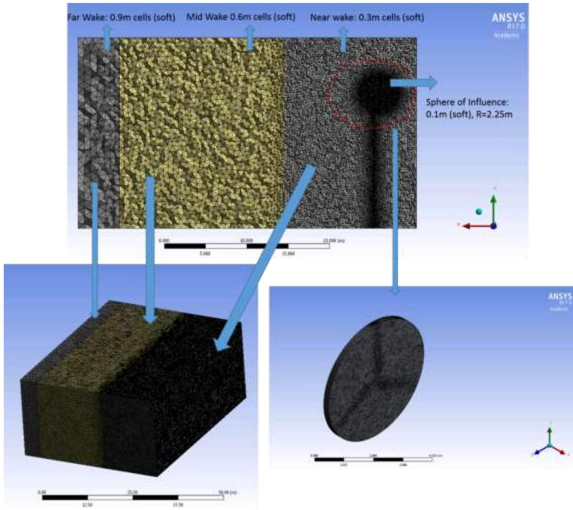
Figure 5.4 – Detailed overview of the mesh sizing procedure.
