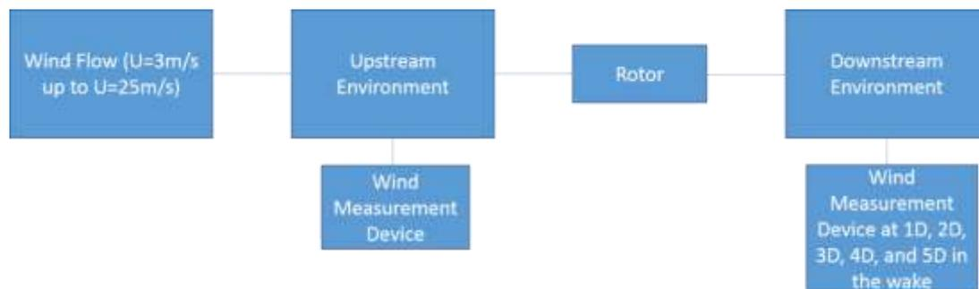
Figure 1.2 - Functional Decomposition Diagram.
