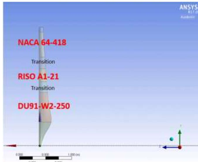
Figure 2.2 - MEXICO rotor geometry, a three-bladed rotor with 4.5m diameter. Source for the blade geometry: Scheppers et al<sup>11</sup>.
