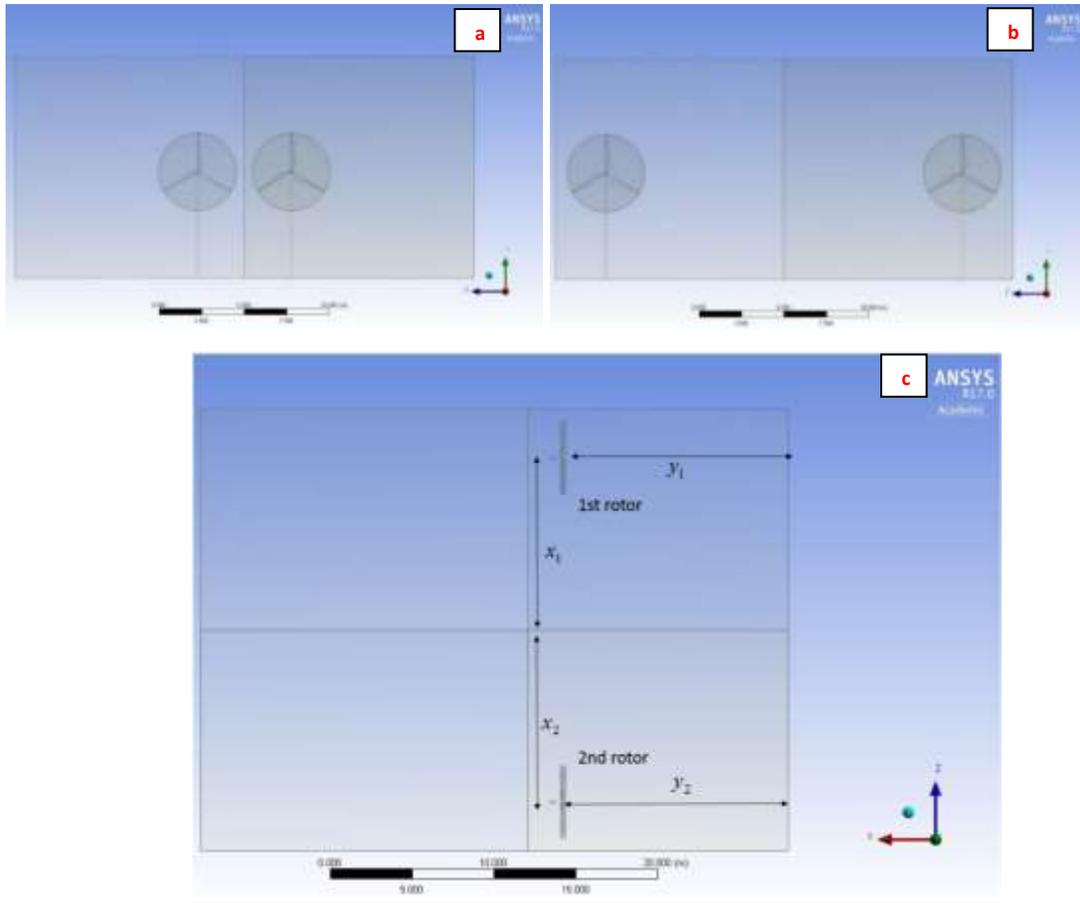
Figure 4.6a and 4.6b: Front view of the lower boundaries for the optimization function; Figure 4.6c: Top view of the physical domain showing each rotor location, and the area occupied by each of them as a function of x and y coordinates.
