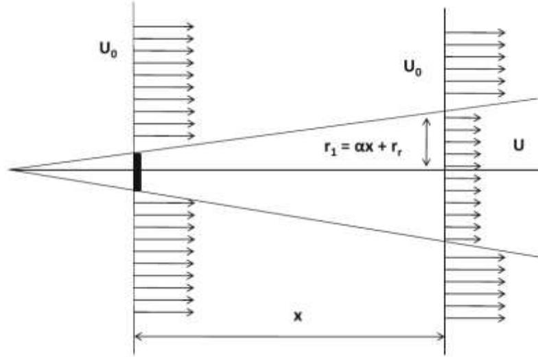
Figure 1.1 - Representation of the wake effect<sup>2</sup>. The black rectangle in the left represents the wind turbine.
