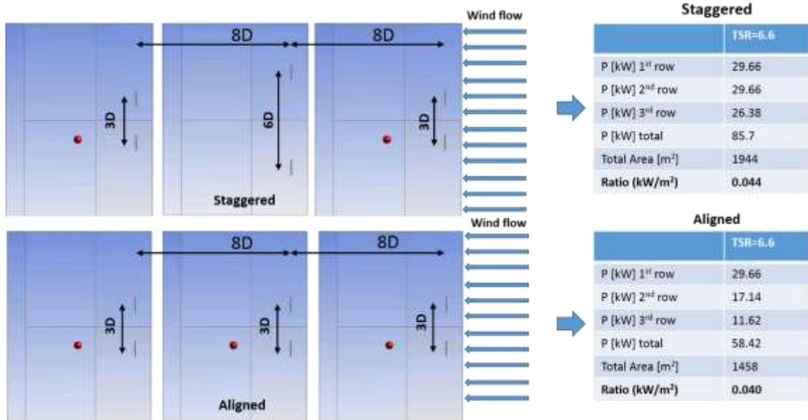
Figure 4.9 - Comparison between staggered and aligned configurations.
