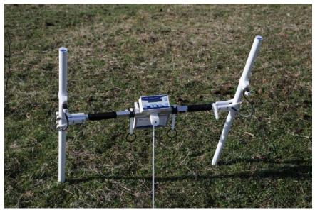
Figure 3.8: The magnetometer survey was performed with a Bartington Grad601 Single Axis Magnetic Field Gradiometer.
