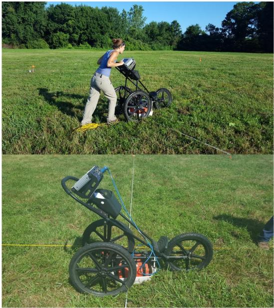
Figure 3.13: Ground-penetrating radar survey conducted by Maeve Herrick and Jasmine Saxon (top) with a 400 MHz antenna and a GSSI 3000 control system (bottom).
