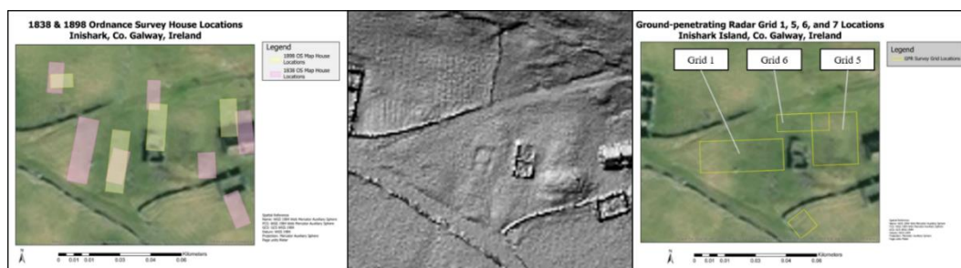
Figure 7: A comparison of building locations on 1838 and 1898 Ordnance Survey maps (left) and LiDAR map data (center) helped select ground-penetrating radar (GPR) survey grid locations. The locations of GPR survey grids 1, 5, and 6 are shown on the modern landscape (right). Maps produced by author in ArcGIS Pro.
