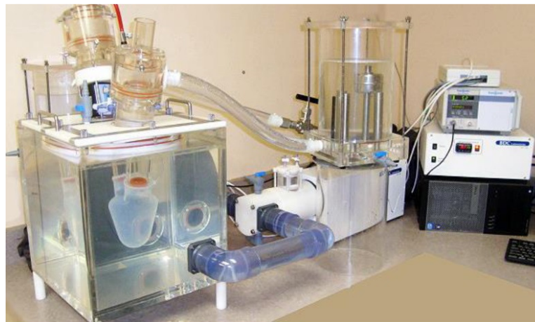
Figure 3.2: Custom-built pulse duplicator system (BDC Labs, Wheat Ridge, CO)
