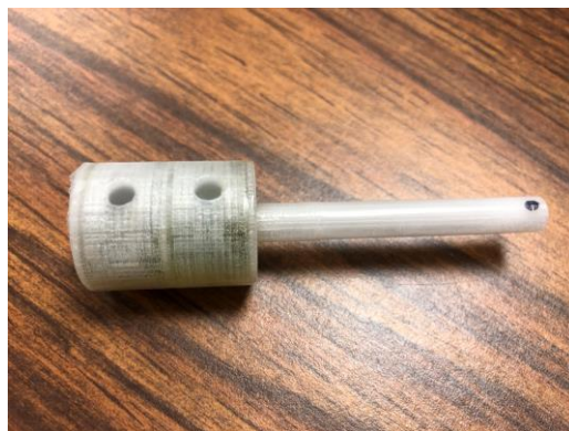
Figure 2.23: 3D printed cylinder sample holder used for L-band imaging experiments. Each chamber was filled with 0.2 mM OX63. A 2 mm divider separates the cylinder into two equal compartments along the Z axis.
