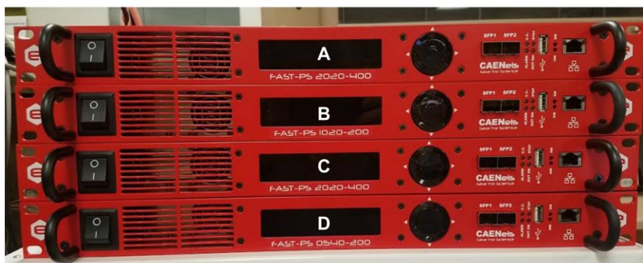
Figure 3.15: CAEN power supplies. (A) X-gradient power supply. (B) Z-gradient power supply. (C) Y-gradient power supply (D) main magnet ( B_0 ) power supply.
