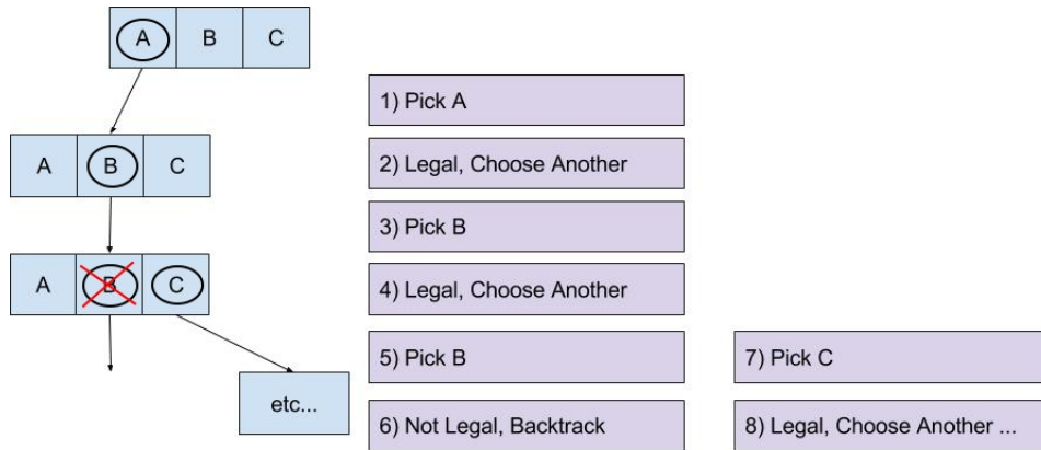
Figure 3.11: Tree Walk Example, Possible notes are A, B, C and rules are no repeated notes
