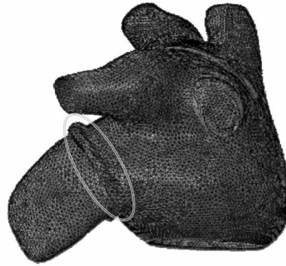
Fig 5.4: Undeformed geometry of the patient-specific finite element model. The encircled region is the ostial entrance to the left atrial appendage.
