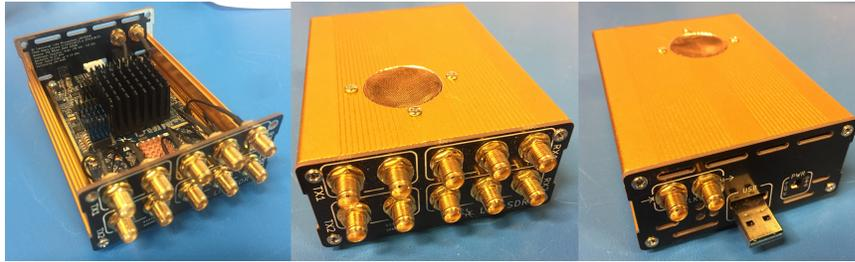
Figure 3.14: LimeSDR Housing from left to right: open, frontside, backside
