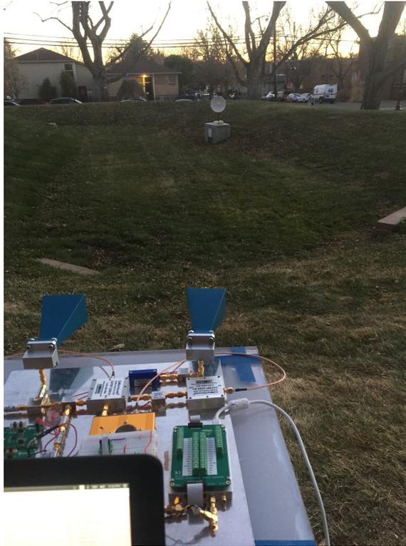
Figure 4.2: X-Band Range Test: Dish target at 20 meters
