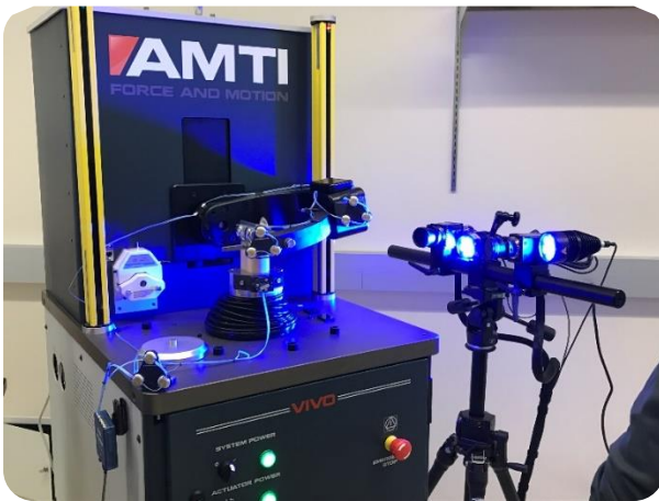
Figure 2-2 AMTI VIVO knee simulator with DIC motion capture system
