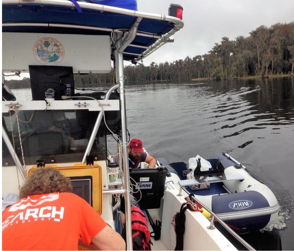
Figure 3.5: Collecting data at Newnan's Lake. The GPR unit is located in the stern of Zodiac Zoom inflatable boat (far right)
