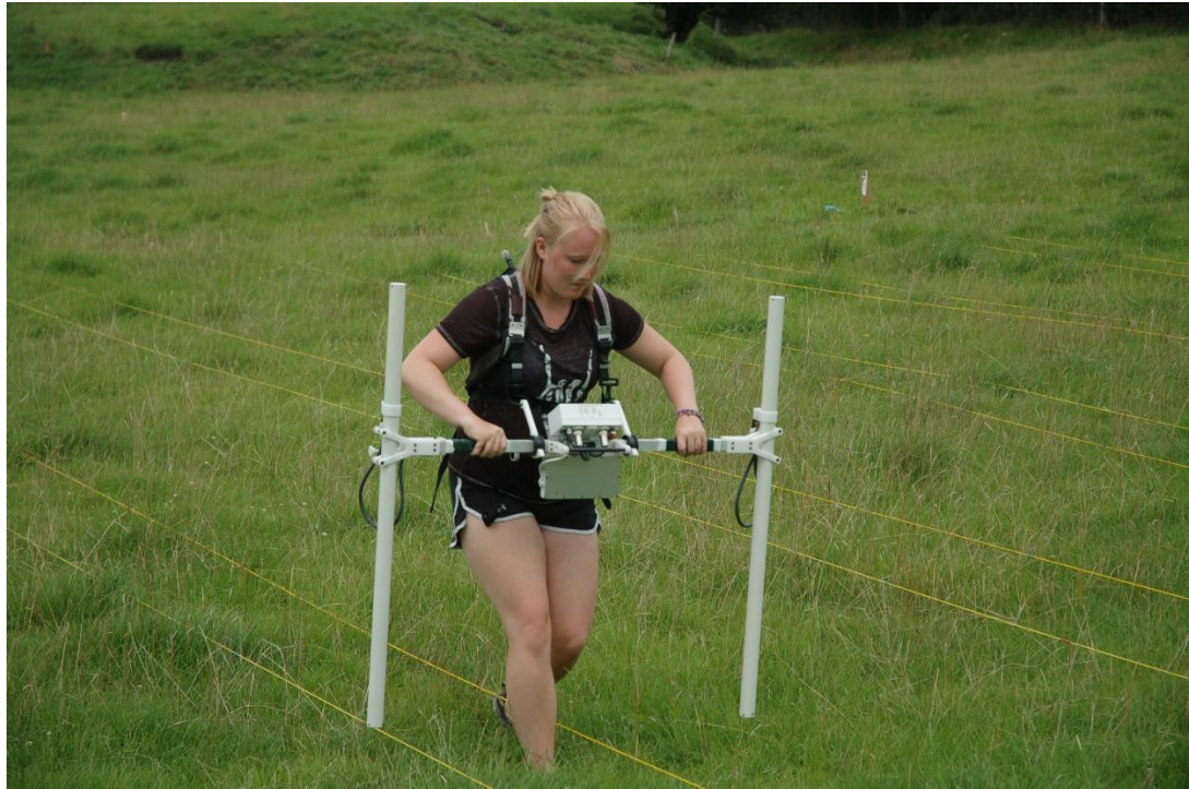
Figure 21: Bartington 601 Single Axis Fluxgate Gradiometer used in the field with transects produced along lines marked with rope (personal photograph).
