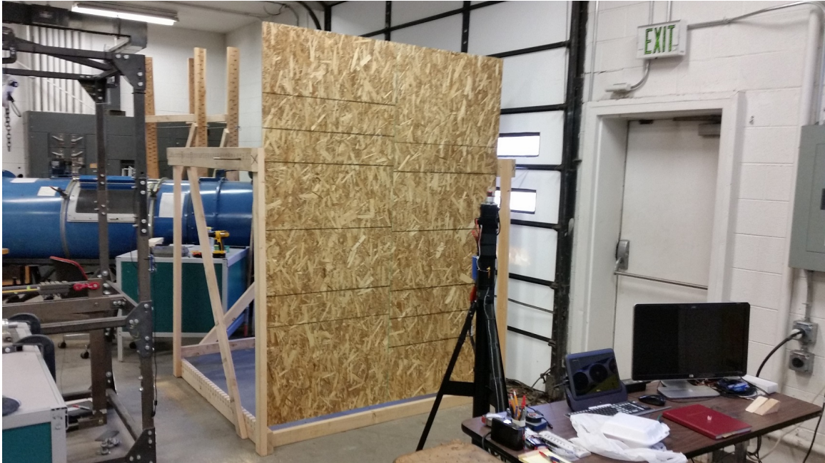
Figure 5.1: Wall effect test apparatus featuring a 8 \times 7 foot OSB plywood wall that can be incremented horizontally from 0 – 60 inches from the test stand.
