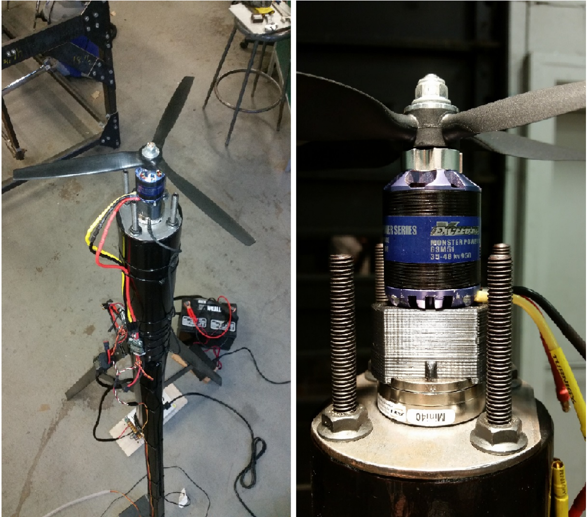
Figure 3.2: Photos of an early test setup using an ExceedRC MonsterPower15 motor with 12 \times 6 3-blade fiber-reinforced composite propeller.
