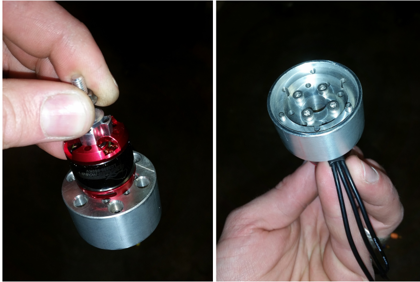
Figure 3.6: Fabricated 45mm aluminum adapter for single Leopard LC2830-980KV Motor and ATI Mini-40 F/T sensor.
