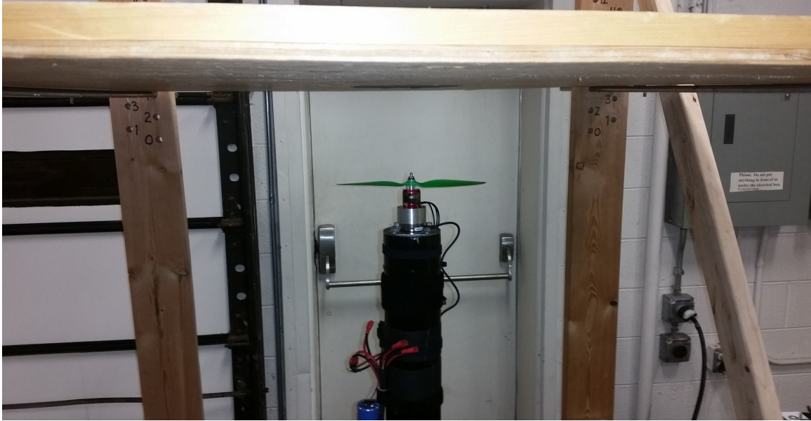
Figure 4.1: Experimental setup for a single isolated propeller, shown at a distance of Z = R from the ceiling surface.
