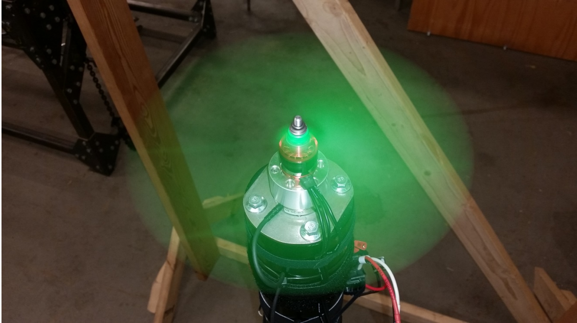
Figure 3.7: Leopard LC2830-12T Motor and GemFan 9 \times 4.7 nylon propeller in single-rotor operation.
