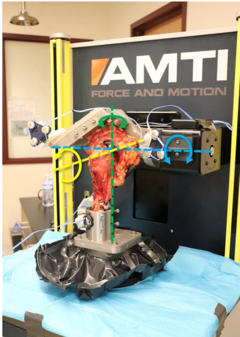
Figure 3.2: A specimen dissected down to the hip capsule cemented into custom fixtures and mounted into the VIVO joint motion simulator (AMTI, Watertown, MA). Primary axes of rotation flexion/extension (yellow), adduction/abduction (blue) and internal/external rotation (green) are labeled.
