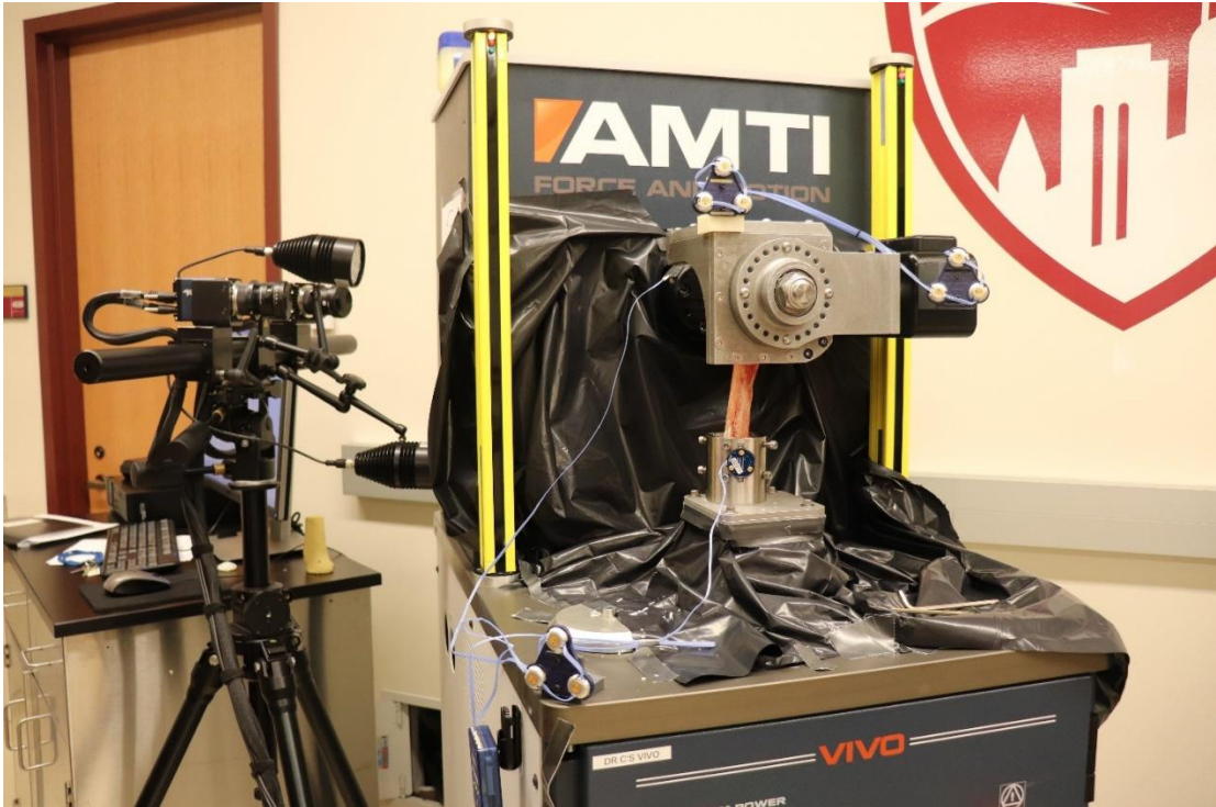
Figure 1.1: The AMTI VIVO (AMTI, Watertown, MA) a 6 DOF joint motion simulator, interfaced with custom fixtures capable of mounting cadaveric hips.
