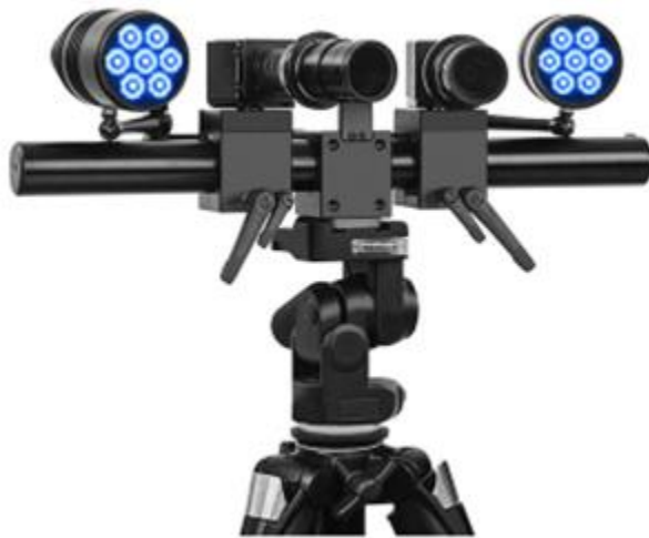
Figure 1.2: GOM Aramis DIC Camera System (GOM mbh, Braunschweig, DE).
