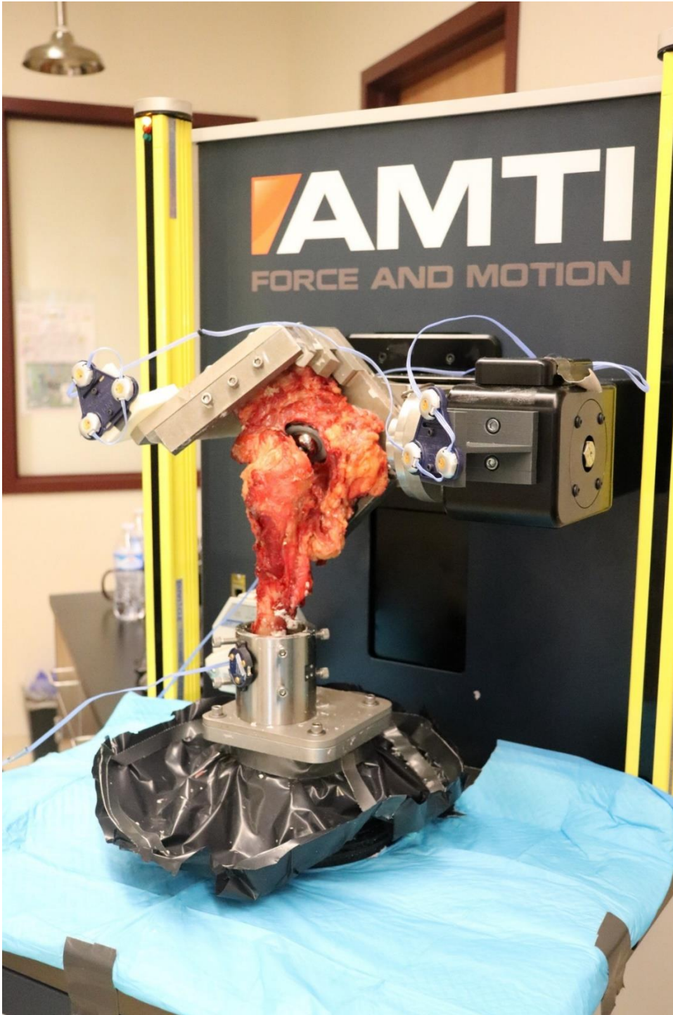
Figure 4.1: A posteriorly-approach implanted Total Hip Replacement (THR) with a pinnacle cup and summit stem mounted into the AMTI VIVO (DePuy Synthes, Warsaw, IN).
