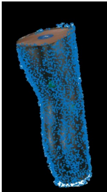
Figure 3.8: Laser scanner point cloud of phantom shank aligned with Kinect Azure point cloud (blue dots) of phantom shank
