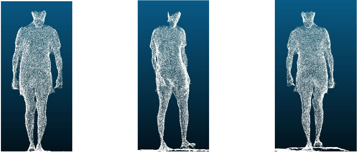
Figure 4.7: Frontal (left), side (middle), and posterior (right) view of the result of the custom program yielding a 3D point cloud from four Kinect Azure cameras
