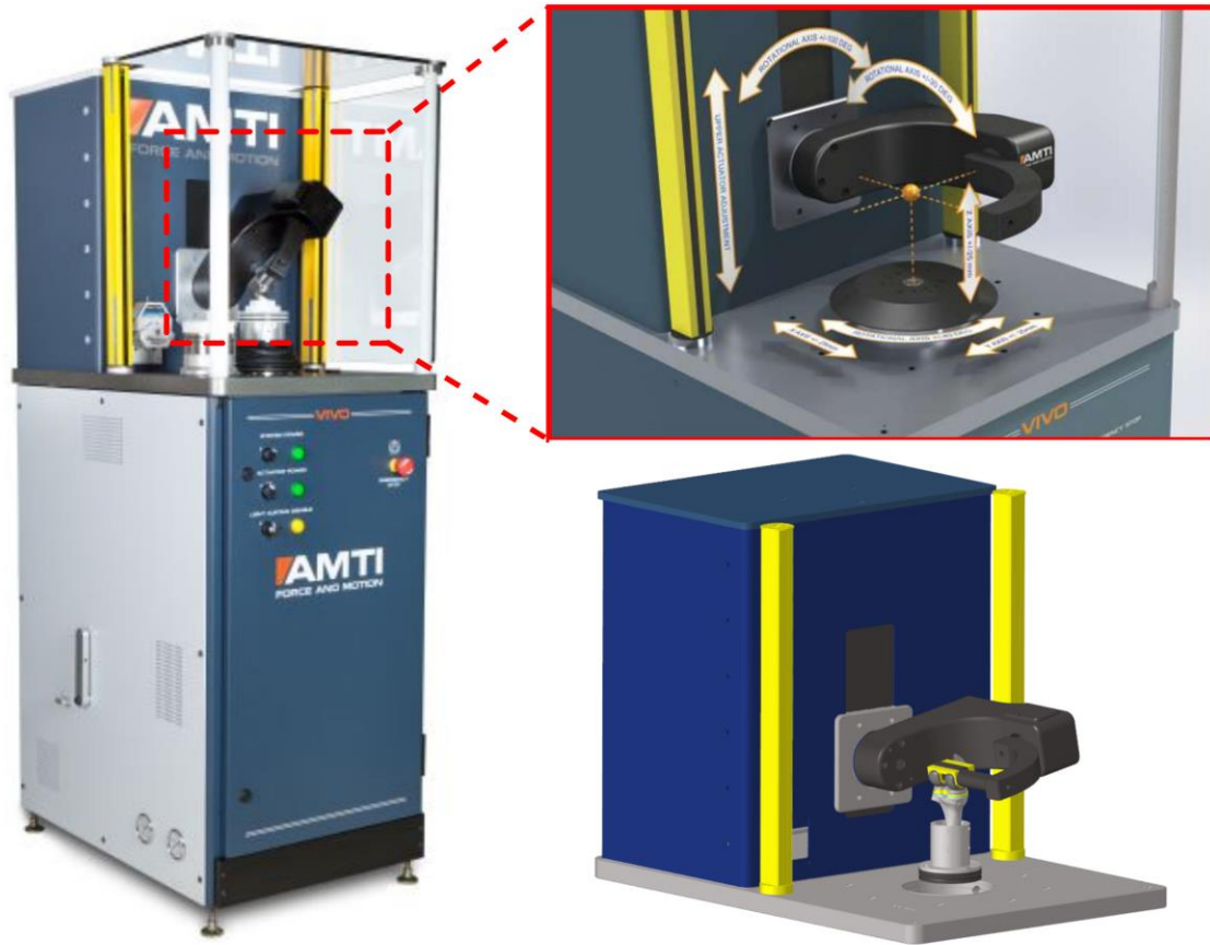
Figure 2.1: The AMTI VIVO™ knee simulator (left) and its validated computational model (right-bottom) (Fitzpatrick et al., 2016). The upper stage can apply flexion-extension and varus-valgus motions/loads, and the lower stage can apply internal-external, superior-inferior, anterior-posterior, and medial-lateral motions/loads.
