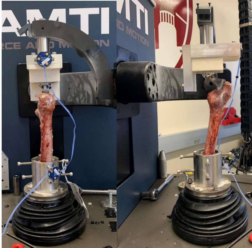
Figure 4.2 Micromotion testing fixture setup in the AMTI VIVO.
