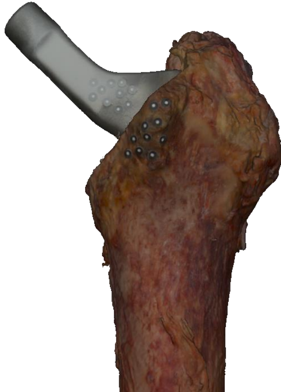
Figure 4.1 Optical Scan of specimen with DIC stickers applied to femoral stem and femur bone.
