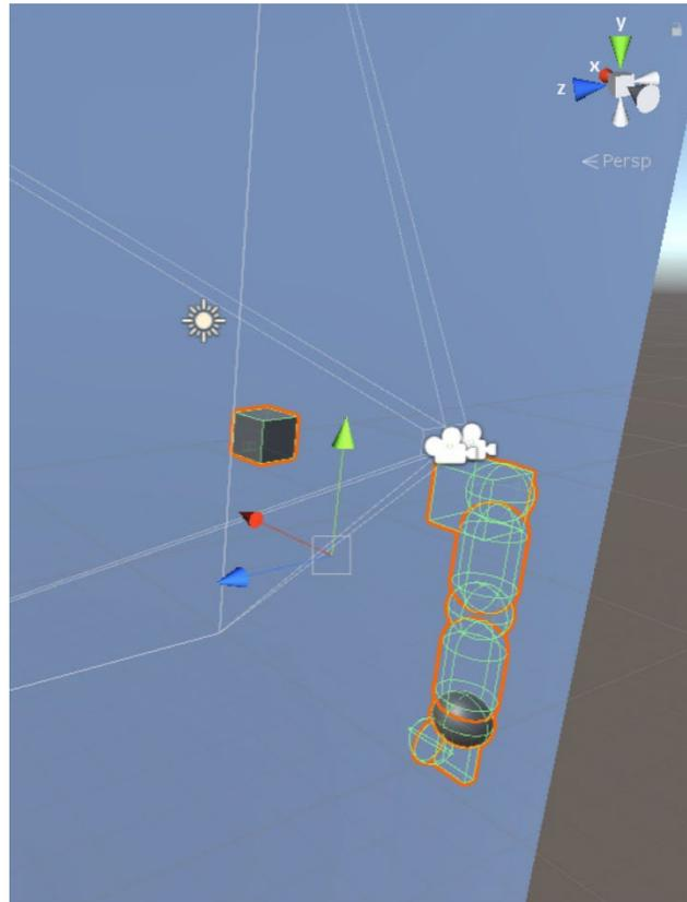
Figure 33: Simulation environment in Unity3D. The axes indicated by the green and the red arrows are aligning with the axes marked by joint 2 and joint 0 in Figure 30, respectively. The blue arrow is pointing inward the shoulder while joint 1 in Figure 30 is pointing outward the shoulder.
