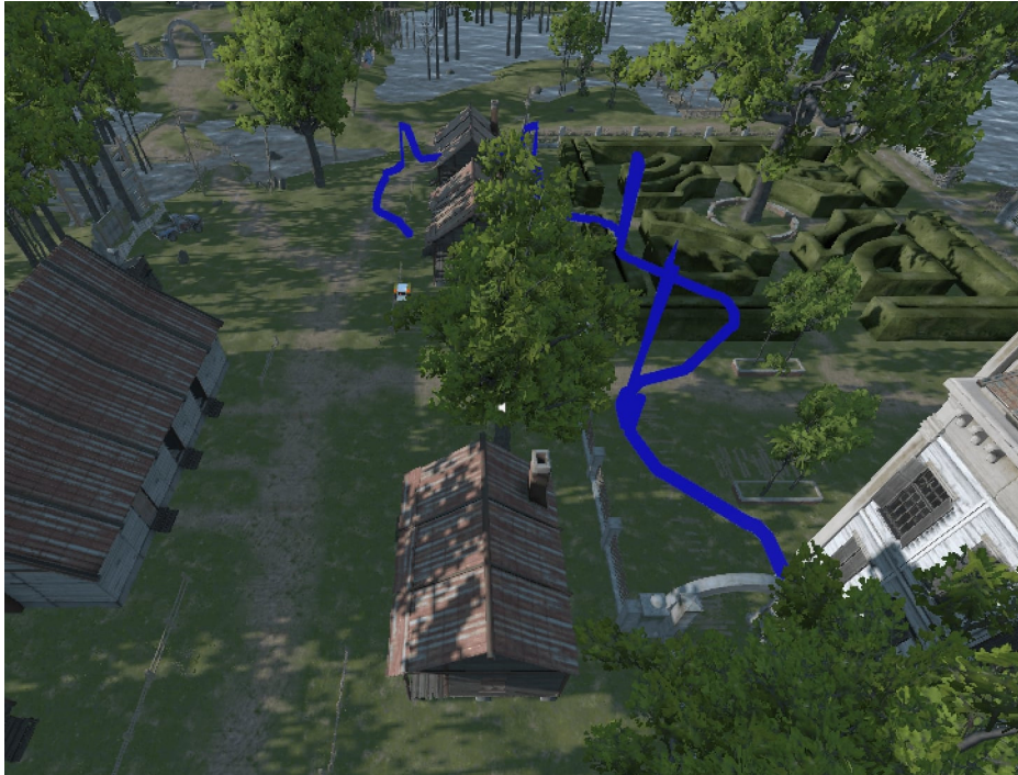
Figure 5.5: Path generated by the global planner to goal position based on the PbIRL concealment costmap
