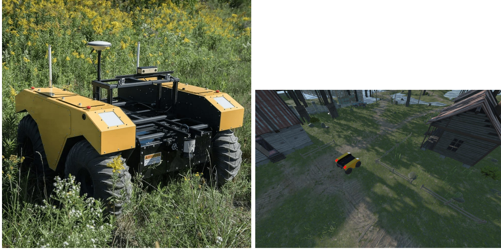
(a) Clearpath Warthog Unmanned Ground Vehicle Robot in a real world field (b) Warthog robot in the simulation environment
