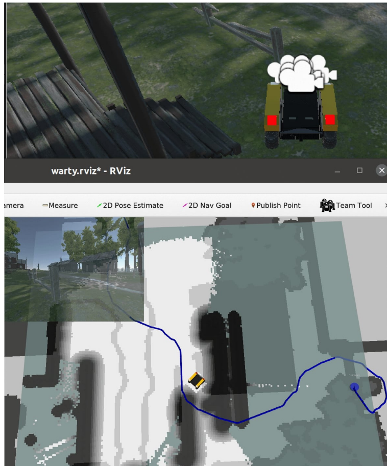
Figure 5.3: Collision of the robot in navigating based on the PbIRL traversability costmap
