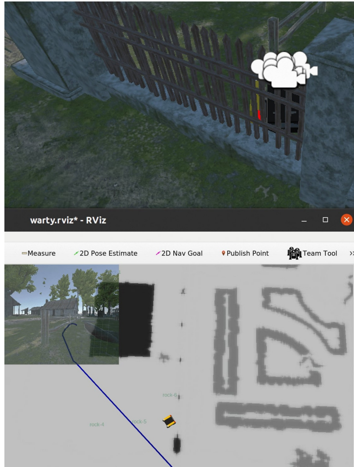
Figure 5.2: Collision of the robot in navigating based on the IOC traversability costmap
