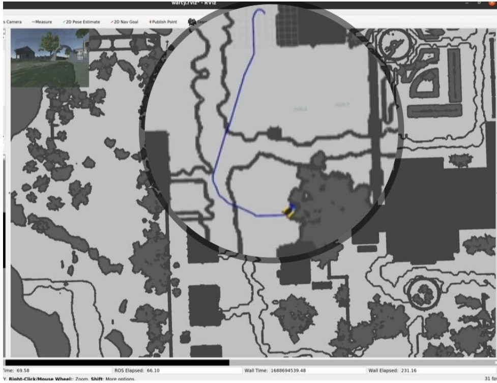
Figure 5.1: Path robot navigated through from the start position to the goal position based on the PbIRL traversability costmap
