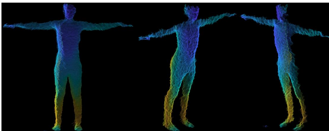
Figure 3.3 The view from the master camera of S01 and the depth image created from aligning the master and subordinate depth data.
