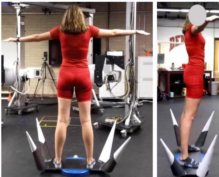
Figure 3.10 A subject standing in the rotated position for the full point cloud collection: facing away from the master camera with the subordinate camera viewing the right side.
