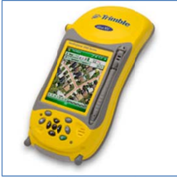
Figure 2: Trimble GeoXH Handheld GPS (Trimble, 2010)
